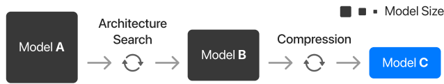
Figure 1: Practitioners start with a feasibility model (A), which is a model of any size that demonstrates that the ML task works. Next, an architecture search looks for a smaller model that is equivalent to (A) and suitable for devices (B). A team decides a budget based on how much more efficient model (B) must be to deploy. Practitioners use techniques to compress their model (B) to reach the budget (C).
